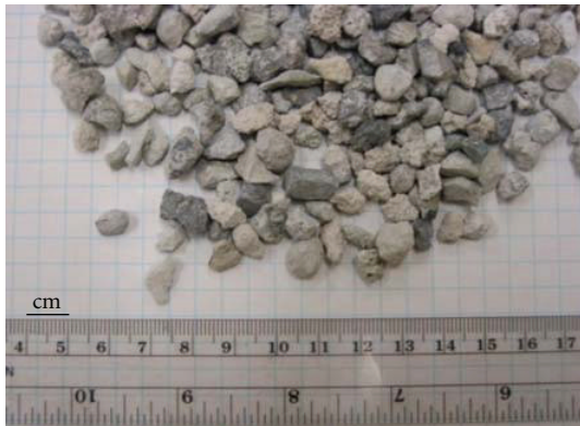
FIGURE 9: Gravel-size EAF(L) slag particles.
