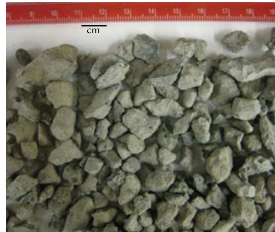
FIGURE 6: Gravel-size BOF slag particles.
