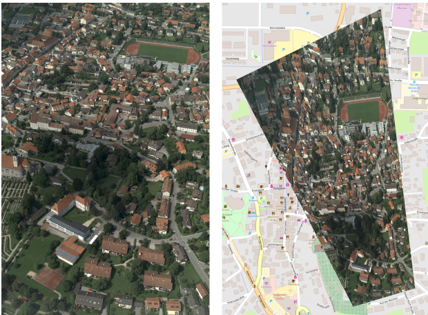
Figure 4. Projective mapping: aerial image and its perspective projection by application of corresponding transformation matrix
