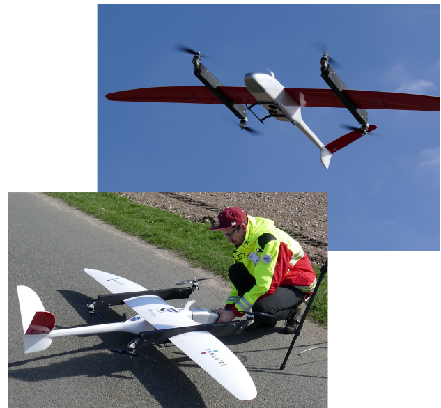
Figure 5. VTOL-UAV Songbird by Germandrones with DLR MACS UAV aerial camera system.
