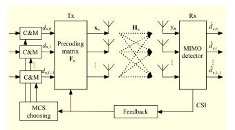
Fig. 1. Illustration of MIMO system over *n*-th subcarrier.
