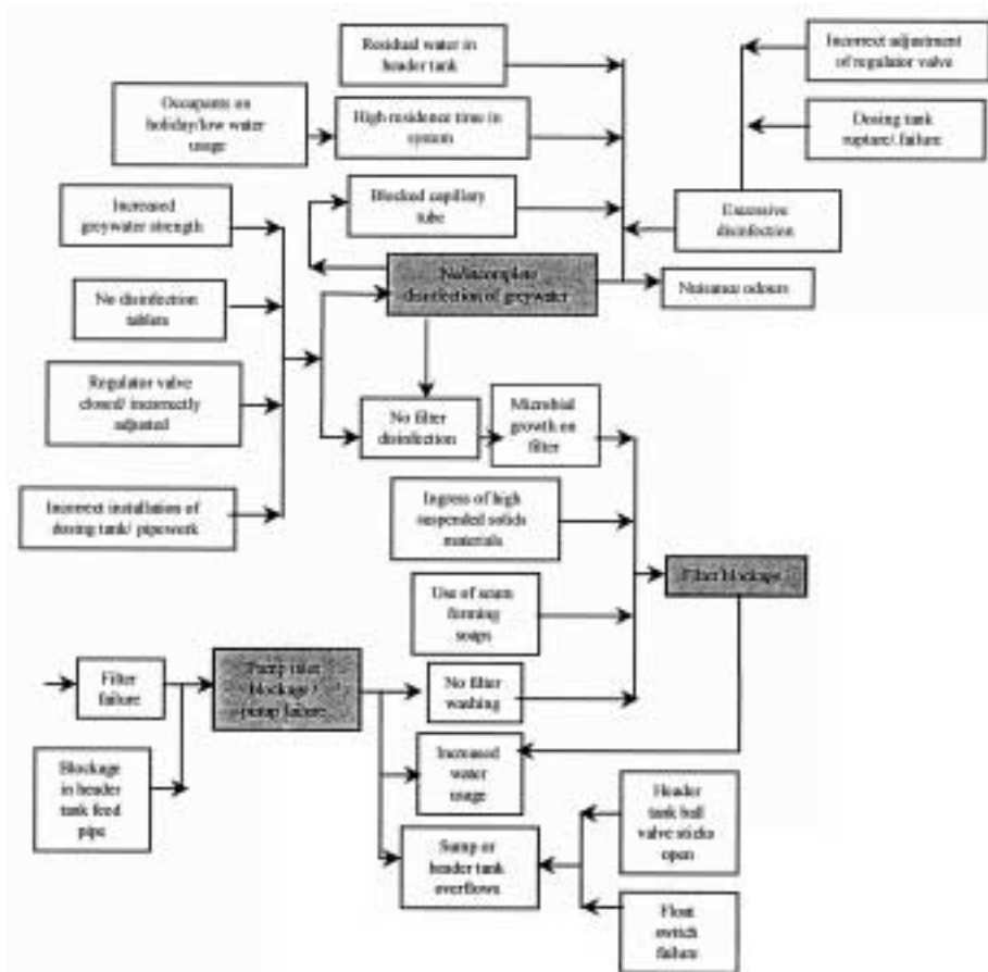
Figure 4 Schematic of HAZOP consequences/causes resulting from deviations in operation of single house greywater recycling system
