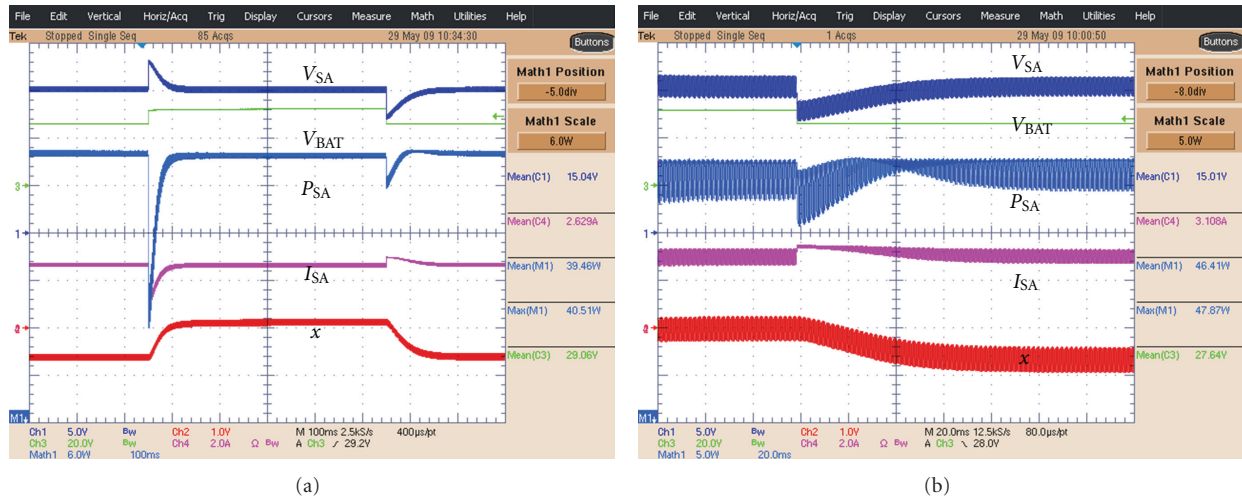
FIGURE 8: (a) Transient waveform when voltage pulse signal is added to battery voltage. (b) Detail of the transient waveforms during a decrease step of the battery voltage.
