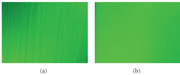
FIGURE 3: Nomarski microscope images of the transferred III-V surface at bonding temperatures of (a) 600^\circ\text{C} and (b) 300^\circ\text{C} .
