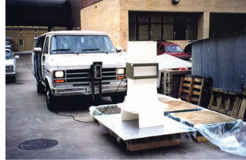
FIGURE 3: Ground penetrating radar and box test sample.
