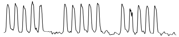
Figure 5: The first three weeks of the power demand dataset. Note the repeating pattern of a strong peak for each of the five weekdays, followed by relatively quite weekends
