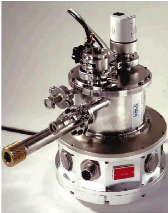
Figure 4.5: Continuous flow cryogenic system (CFC), that keeps the detectors cooled by a continuous flow of liquid nitrogen, which surrounds the CCDs. CCDs used in astronomy must operate in the temperature range between 140 and 160 K. (Dorn et al., 2000).
