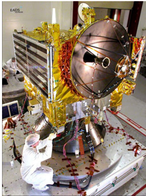
Figure 3.8: The Venus Express : final payload assembling procedures. (image: ESA's Venus Express mission website).
