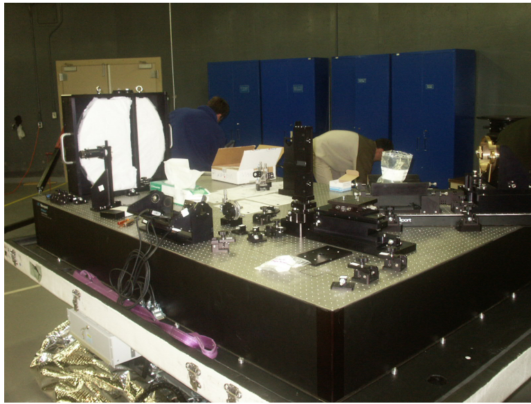
Figure 5.2: High resolution spectrograph and spectropolarimeter ESPaDOnS. (Image from CFHT official website)
