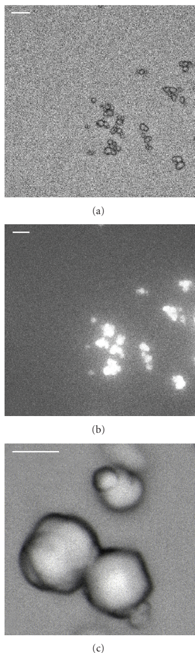
FIGURE 3: Microscope images of MCM-DPA sample, (a) and (b) reflected and emitted light, respectively, from silica particles on glass substrate and (c) software-assisted zoom, showing silica powder morphology (scale bars 10\ \mu\text{m} ).
