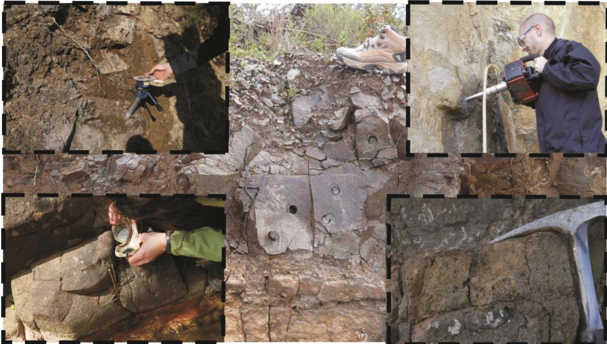
Figure 4: Field pictures from the Algarve basin's outcrops. The magnetic and solar compass and the driller used to collect the samples (at the top). Inclinometer and the hammer used to mark the separation between two different lava layers, useful to estimate bedding corrections (at the bottom).
