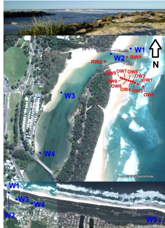
Figure 2. Instrument locations in Mooball Creek. Numbers of pressure sensors and stilling wells. Blue: filed trip 1; Red: field trip 2,
