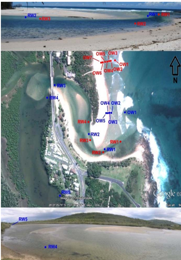
Figure 1. Instrument locations in Cudgera Creek. Numbers of pressure sensors and stilling wells. Blue: field trip 1; Red: field trip 2;
