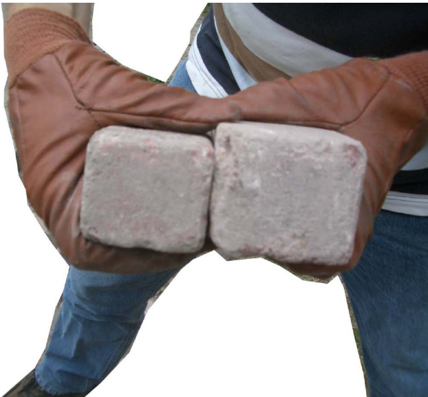
Figure 103. Bricks at Kennedylaan, Heerenveen, 2007 Peter Wouda demonstrating two common bricks, notably the 200 x 150 x 100mm module on right.
