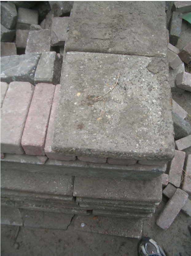
Figure 104. Pavers at Kennedylaan, Heerenveen, 2007 Often 300 x 300 x 45mm pavers are used as a cap or to tie across brick courses.
