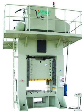
Figura 12 – Single Action Presses
