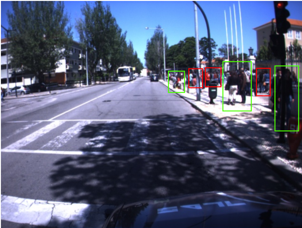
Figure 4.3: Ground truth example 2 - Occluded pedestrians that stand in close or medium range are also valid targets.
