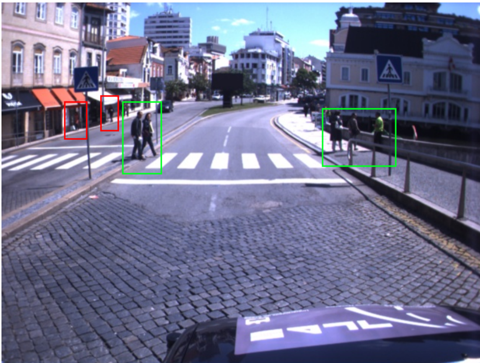
Figure 4.6: Ground truth example 5 - Two pedestrians crossing the street together are considered to be one target.
