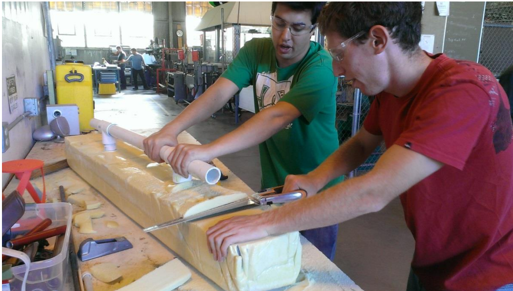
Figure 14: Removal of Extra Foam on Pontoons
