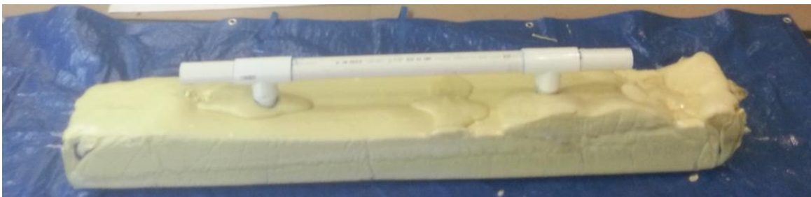
Figure 13: Poured Foam Pontoon after Demoulding
