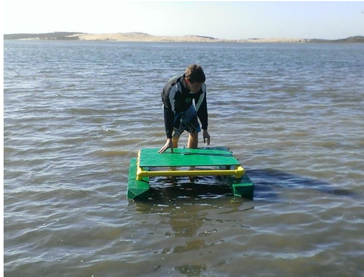
Figure 24: Float and Stability Tests of Raft
