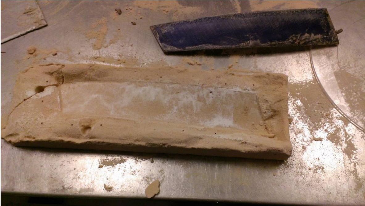
Figure 16: Attempt to Green Sand Cast Full-Scale Turbine Blade Half
