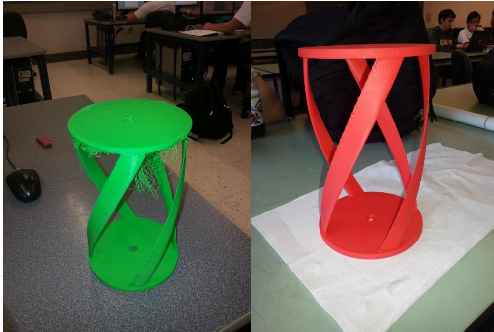
Figure 15: Failed (L) and Final (R) Half-Scale Turbine Rapid Prototypes
