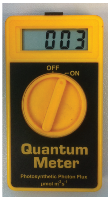
Figure 4. Light-intensity data were collected with a hand-held light meter.
