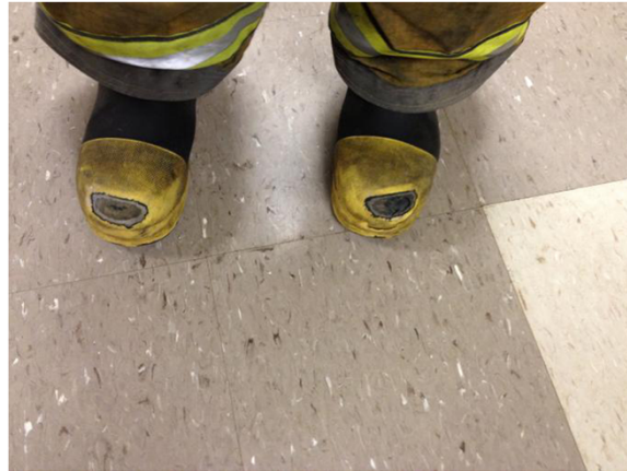
Figure 4 Worn out toe cap due to frequent friction on the ground while crawling.
