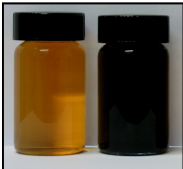
Figure 1 Photograph of graphene oxide (left) and bacterially reduced graphene oxide (right) at a concentration of 500 \mu\text{g/mL} .
