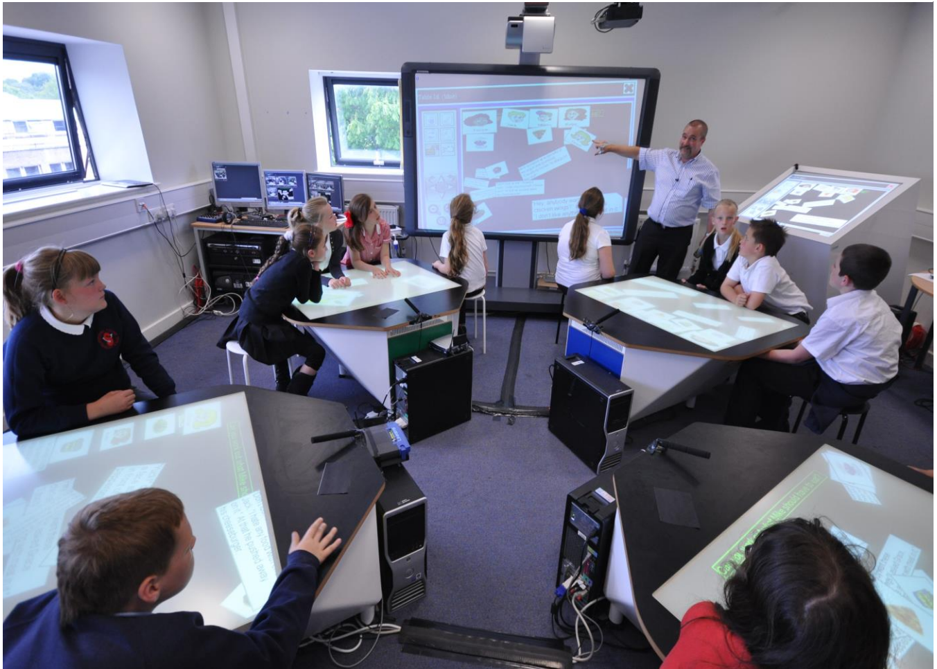
Figure 1.2: The SynergyNet classroom with 4 linked multi-touch tables and the teacher orchestration desk (back right hand corner of the classroom)
