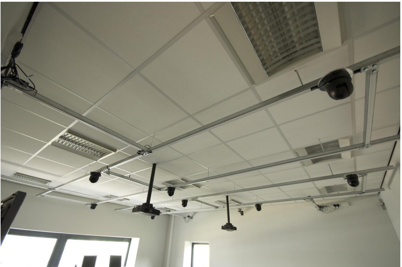
Figure 1.3: The array of cameras to capture data from each of the four tables in the SynergyNet classroom
