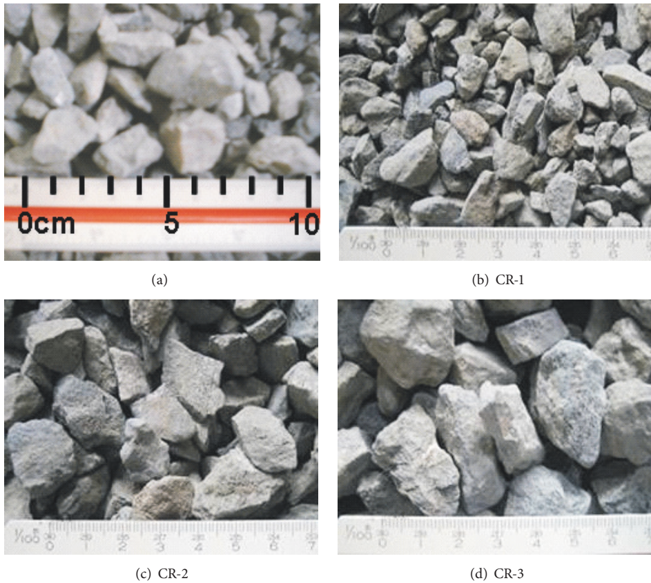
FIGURE 4: Classification of crushed rocks by diameter: (a) mixed sizes of 2–26.5 mm, (b) 4.75–9.75 mm (CR-1), (c) 9.75–14.9 mm (CR-2), and (d) > 14.9 mm (CR-3).
