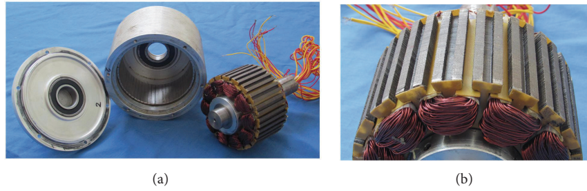
FIGURE 14: Prototype machine. (a) Stator and rotor assembly. (b) FMPs in stator.
