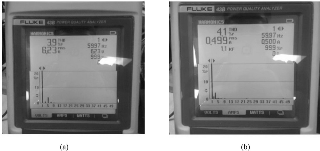
Fig. 13.(a) Practical output voltage THD, (b) Practical output current THD
