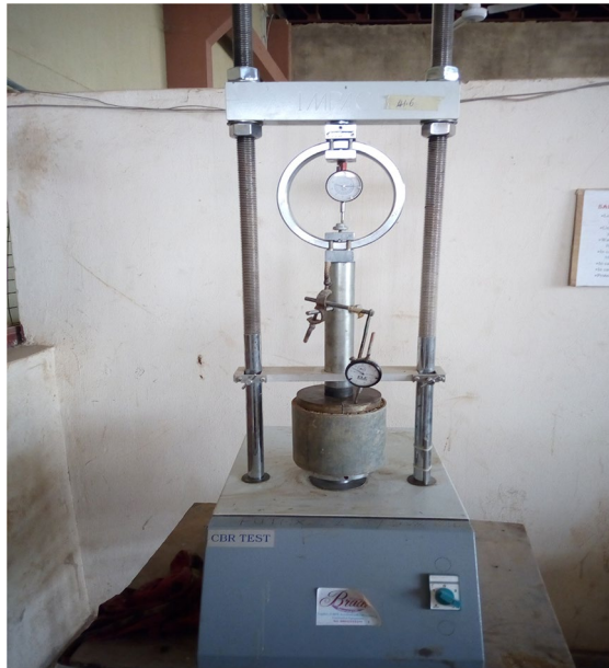
Fig. 4 Laboratory setup for conducting CBR test
