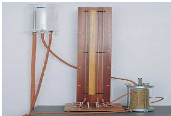
Fig. 5 Laboratory setup of falling head permeameter testing
