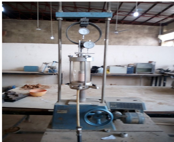
Fig. 3 Triaxial testing setup for unconfined compression test
