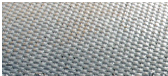
Fig. 2 The woven material of the soft fuel tank
