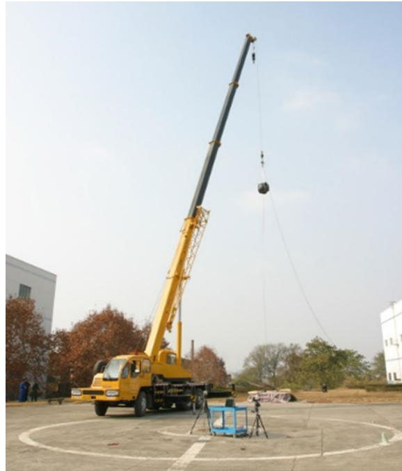
Fig. 4 Experimental facilities of the drop impact test
