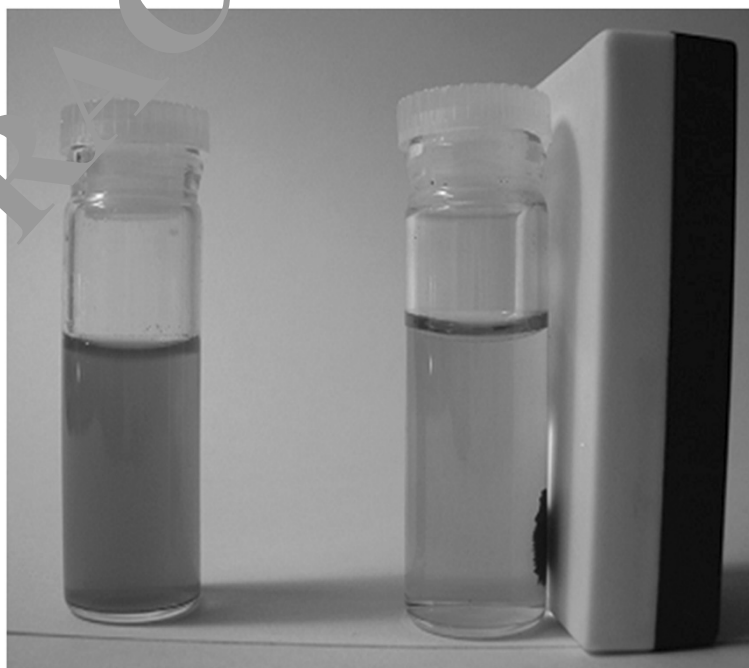
Figure 3 Magnetite-hexane suspension attached to a magnet.
