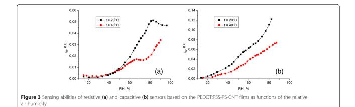
the water molecules, which have large dielectric constant ( $\varepsilon$  = 81) as compared to the silicon. This is why increasing relative humidity of the air causes a noticeable increase of the capacitance of the hybrid nanocomposites PEDOT:PSS-PS-CNT.
