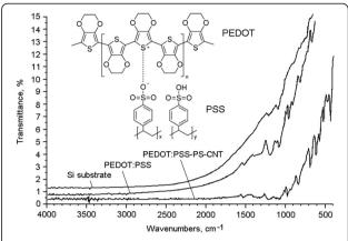
**Figure 1** FTIR spectra of silicon substrate, PEDOT:PSS, and hybrid PEDOT:PSS-PS-CNT films on the silicon substrate. Inset shows chemical formula of PEDOT:PSS.
