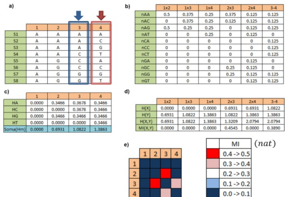
Fig. 3 VMI calculation – the blue and red arrows point to a particular pair (X,Y), but all possible pairs are calculated: a) S1, S2 ... to S8 are aligned sequences versus DNA positions (residues); b) nucleotide relative frequency distribution for all pairs of nucleotides; c) vertical entropy of each residue and at the bottom the vertical entropy per residue; d) mutual information calculation for pair of residues; and e) on the left is the VMI bidimensional spectrum represented as a heat map, and on the right side we see the color scale
