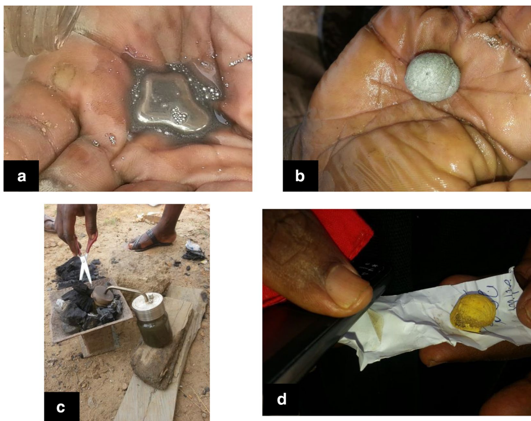
Fig. 3 Crude method of gold processing using mercury by small scale miners. a Mercury being handled by a small-scale miner in the palm; b mixture of mercury and gold ore; c charcoal heating of gold amalgam in retort device; d gold separated from the amalgam
