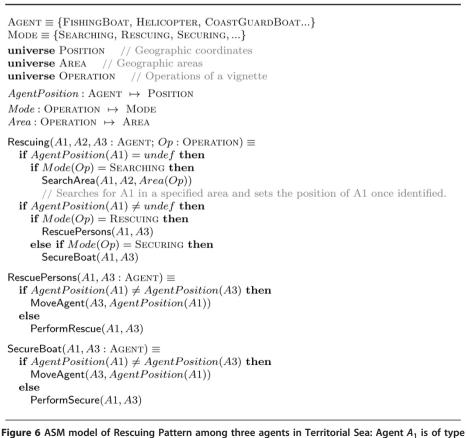
Figure 6 ASM model of Rescuing Pattern among three agents in Territorial Sea: Agent  $A_1$  is of FISHINGBOAT,  $A_2$  is of type HELICOPTER, and  $A_3$  is of type COASTGUARDBOAT.
