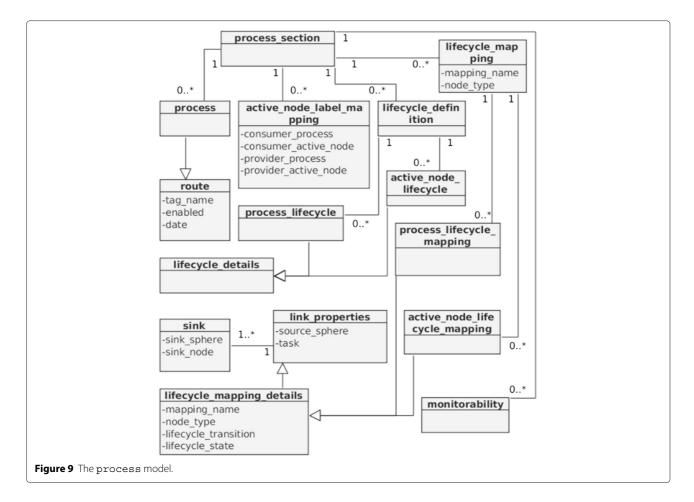
instrumental for defining life-cycle stages of entire processes, or merely active nodes that are part of respective processes. Such definitions are part of consumer- and provider processes. The classes process\_lifecycle and active\_node\_lifecycle are subclasses of lifecycle\_details. The latter class is part of the eSourcing perspective that we explain in the sequel.
