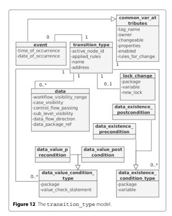
If workflow\_visibility\_range in data is true, a package is visible in all cases of a process template for all active nodes contained. If case\_visibility is true, a data package is visible for all cases.
