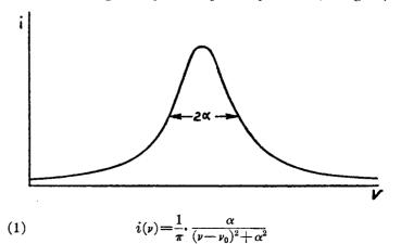
where  $\nu$  is the frequency,  $\nu_0$  the frequency in the middle of the line and  $\alpha$  a constant. The dependence of the line
