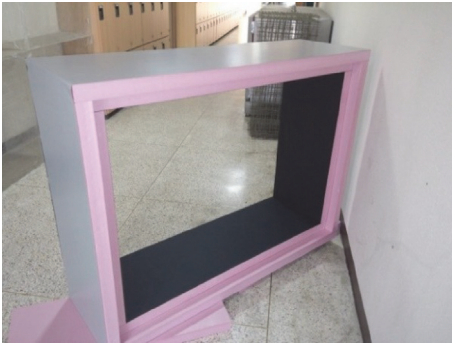
FIGURE 6: Test box configuration for the indoor bifacial BIPV panel with an integrated reflector.
