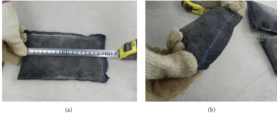
FIGURE 1: Geobag used in the model tests. (a) Measuring the size of geobag; (b) sewing up the geobag.
