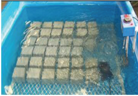
FIGURE 2: Water curing (WAC).
