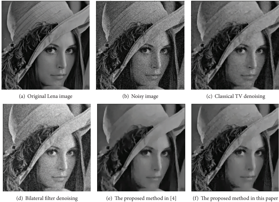
FIGURE 3: Comparison of denoising results by different methods. (The SNR value of this comparison is as follows: noisy image SNR = 7.1122, classical TV denoising SNR = 14.3264, bilateral filter denoising SNR = 14.2720, the proposed method in [4] SNR = 14.6837, and the proposed method in this paper SNR = 14.8013.)
