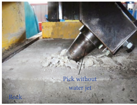
FIGURE 6: Photo of cutting experiment and cutting force for pick without water jet.
