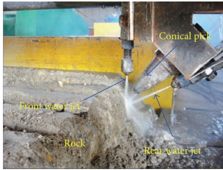
FIGURE 14: Photo of cutting experiment for JFRP.
