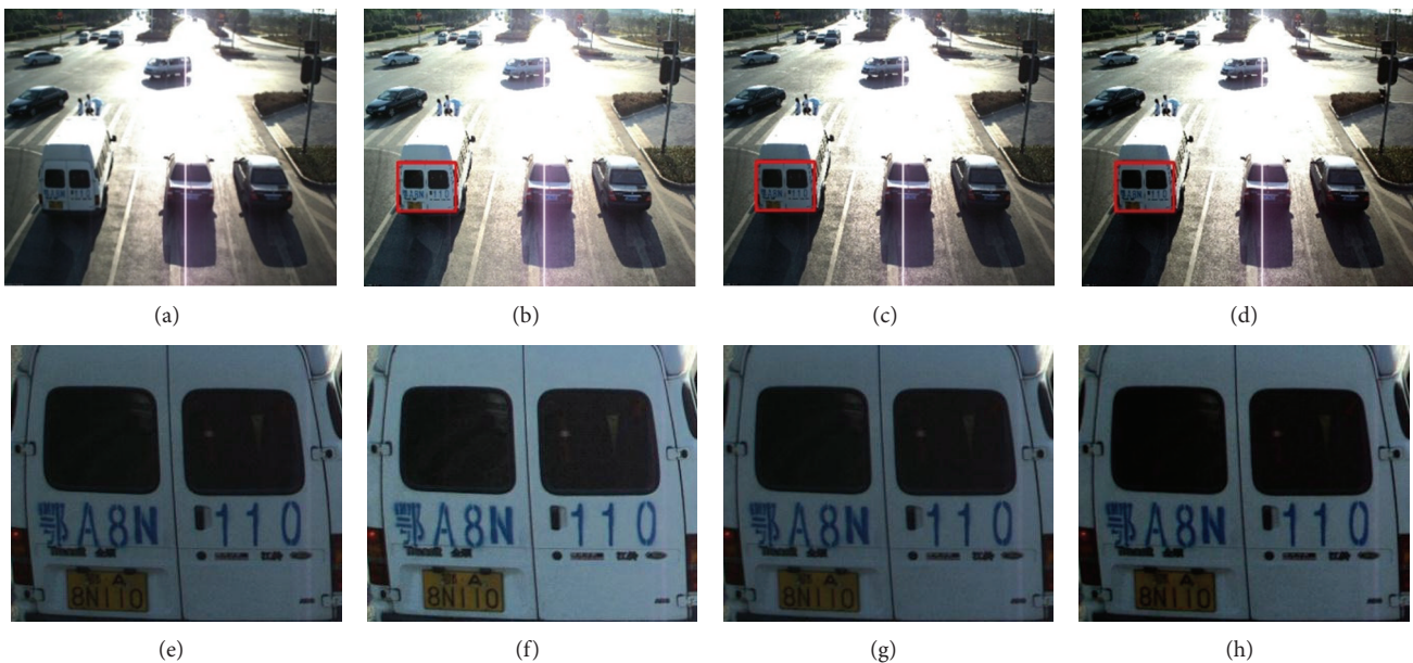
FIGURE 8: Enhancement result for backlight image. (a) Original. (b) Proposed image. (c) Histogram extension image. (d) ESIHE image. (e) Cropped and enlarged results of (a). (f) Cropped and enlarged results of (b). (g) Cropped and enlarged results of (c). (h) Cropped and enlarged results of (d).
