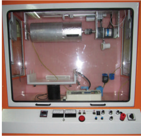
FIGURE 1: The MEP used for nanofiber production by electrospinning [1].
