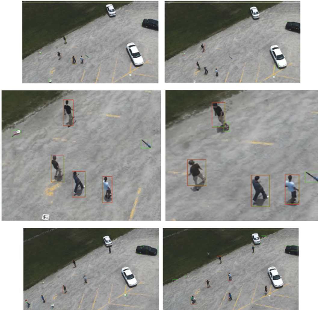
FIGURE 14: Human detection for multiple human with different actions from UCF-ARG dataset: Green boundary boxes in each image are the results after using optical flow. The red boundary boxes are the results after applying human classification based on deep models. The first and third rows are the original frames. The second row is the first row after zooming in on the persons.
