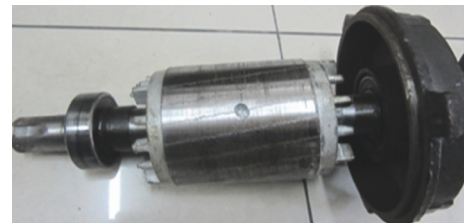
FIGURE 7: The rotor with one broken bar.
