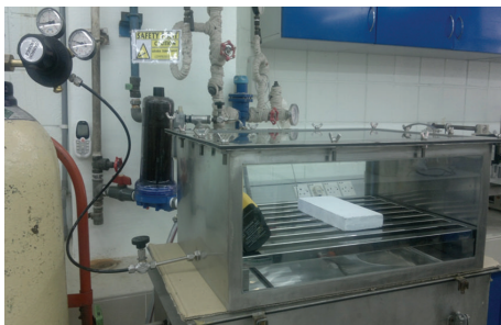
FIGURE 3: LiNbO 3 coated concrete slab in reaction chamber.
