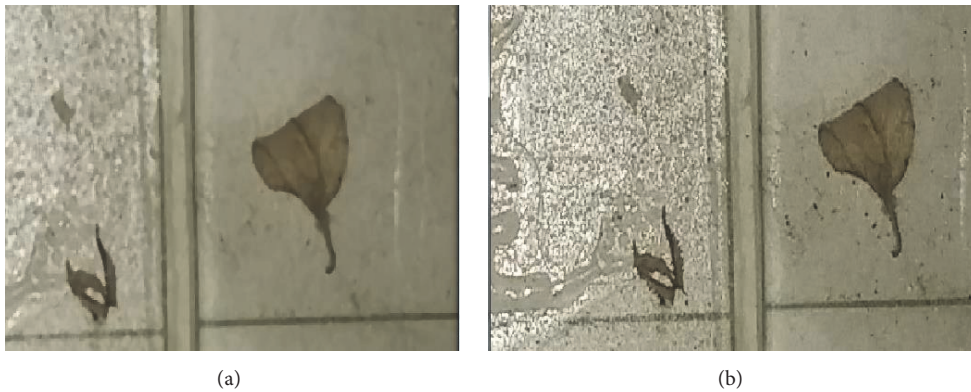
FIGURE 7: (b) The original image, where powder can interfere with the histogram. (a) The processed image with equalization and median filter applied; the dust particles disappear.
