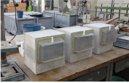
FIGURE 2: Set of specimens with the moisture load arrangement.
