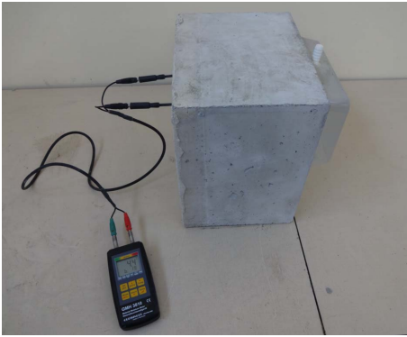
FIGURE 4: Real measurement by the electrical resistivity moisture meter.
