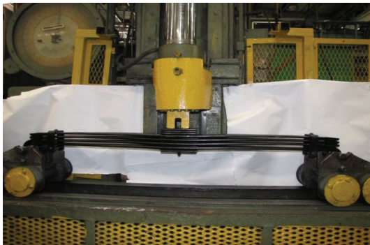
FIGURE 5: Experimental vertical stiffness test for leaf springs.
