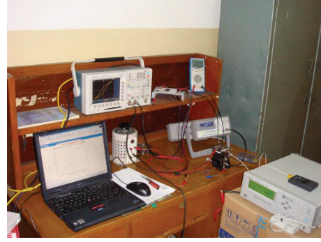
FIGURE 4: P - E and dielectricity characterization system.
