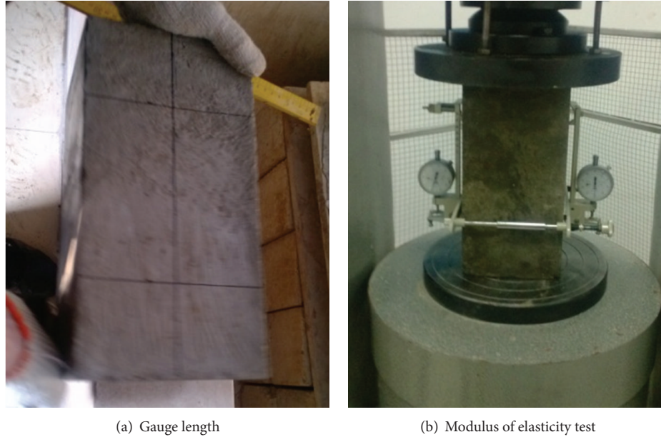
FIGURE 9: Testing arrangement of modulus of elasticity.
