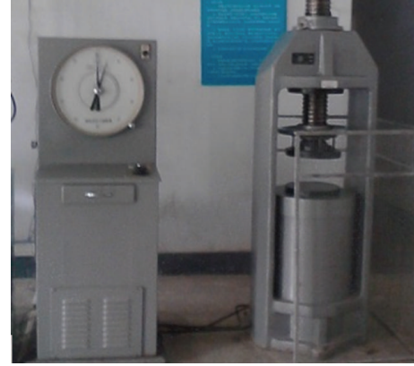
FIGURE 1: Compression testing machine 1 (2000 kN).
