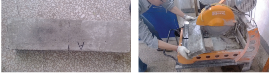
FIGURE 3: Damage simulation of slab using cutting machine.
