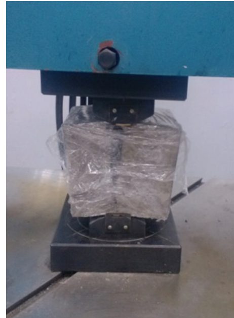
FIGURE 5: Splitting tensile test.
