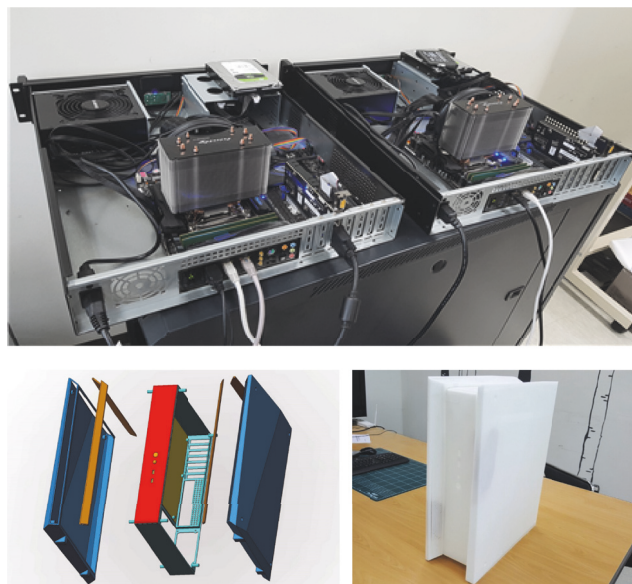
FIGURE 5: H/W prototype and 3D printing product of Abyss storage cluster.
