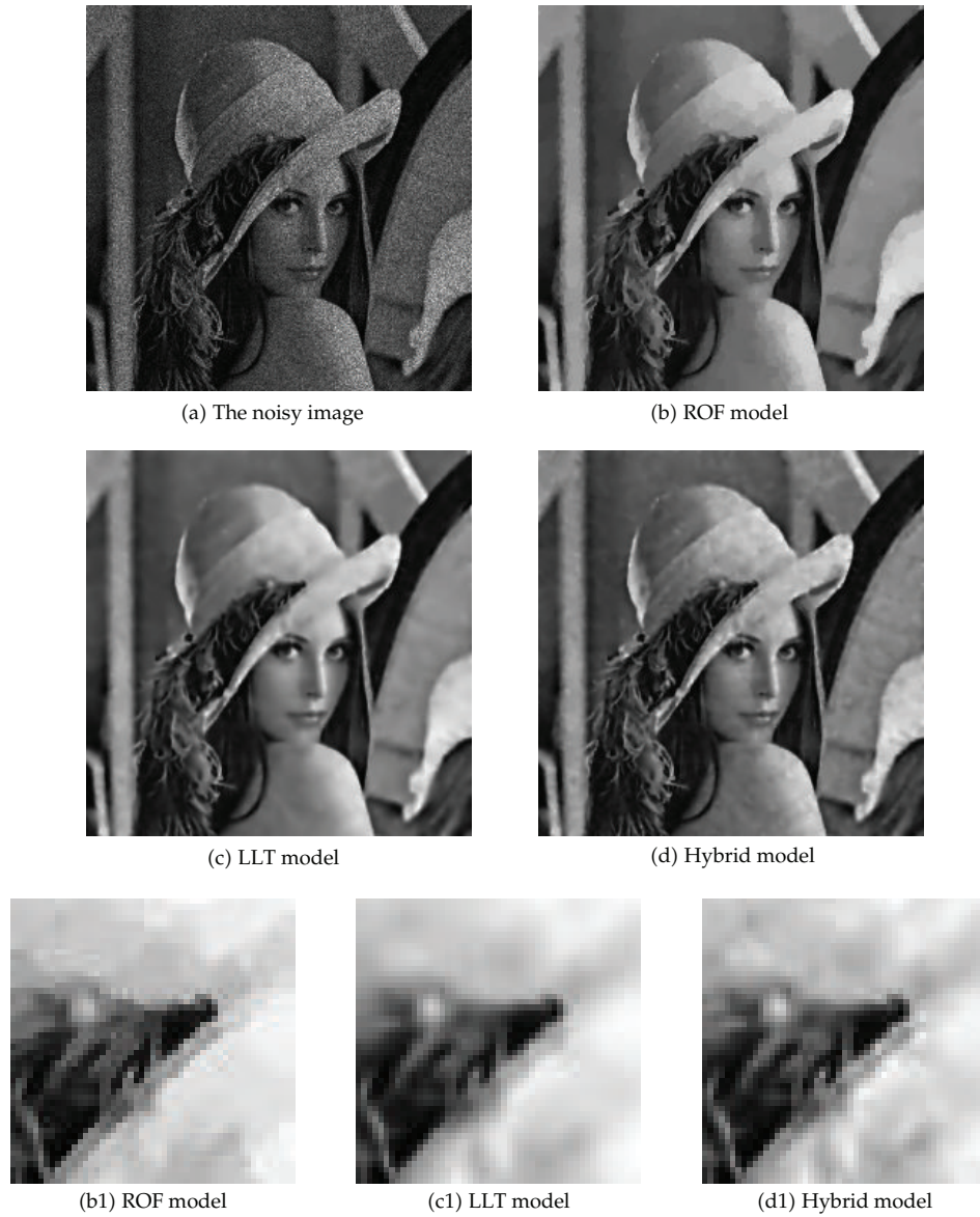
Figure 8: The related images and the local zooming images in Example 4.13. SNRs: (a) 9.2017; (b) 15.6059; (c) 15.1754; (d) 16.0546.
