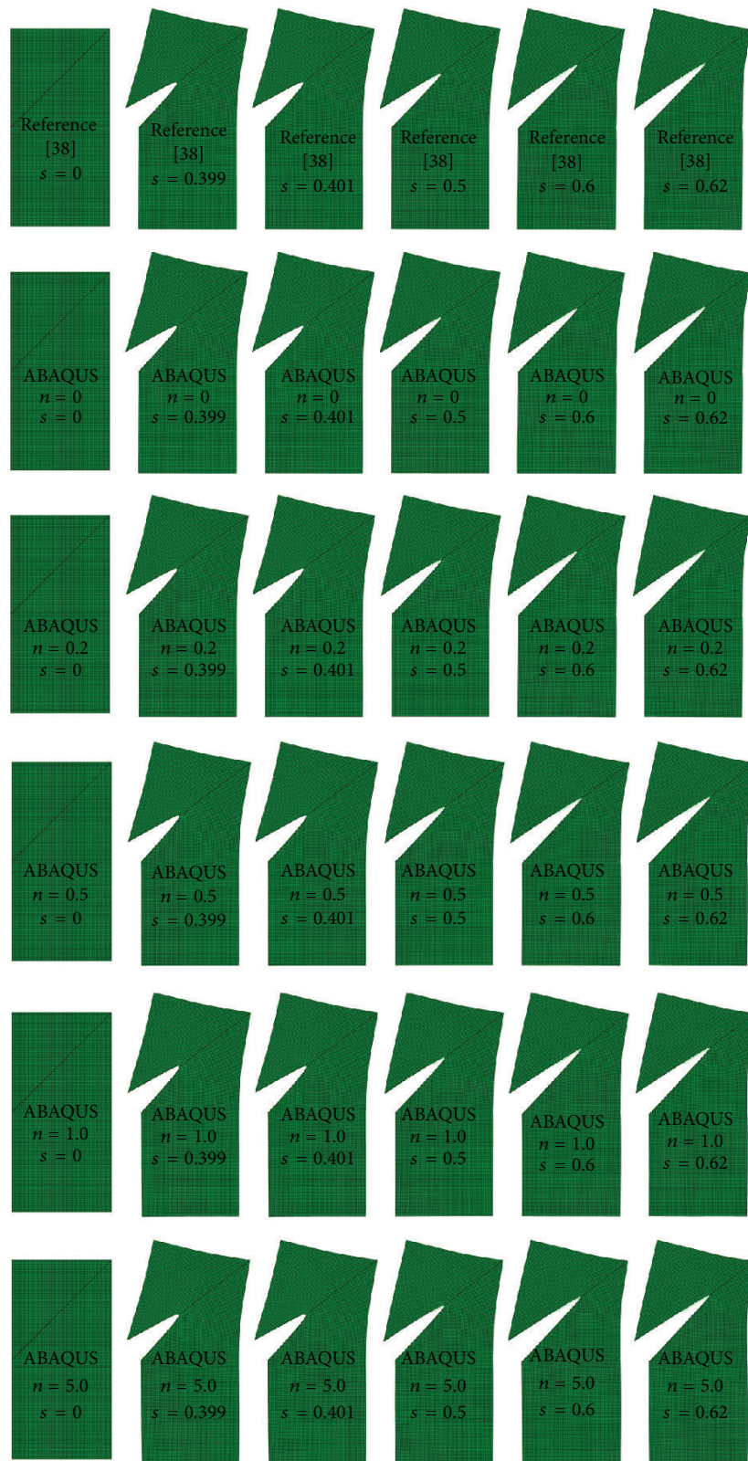
FIGURE 17: Deformed body for dynamic crack propagation at different crack length ( C = 0.2 C_s ).
