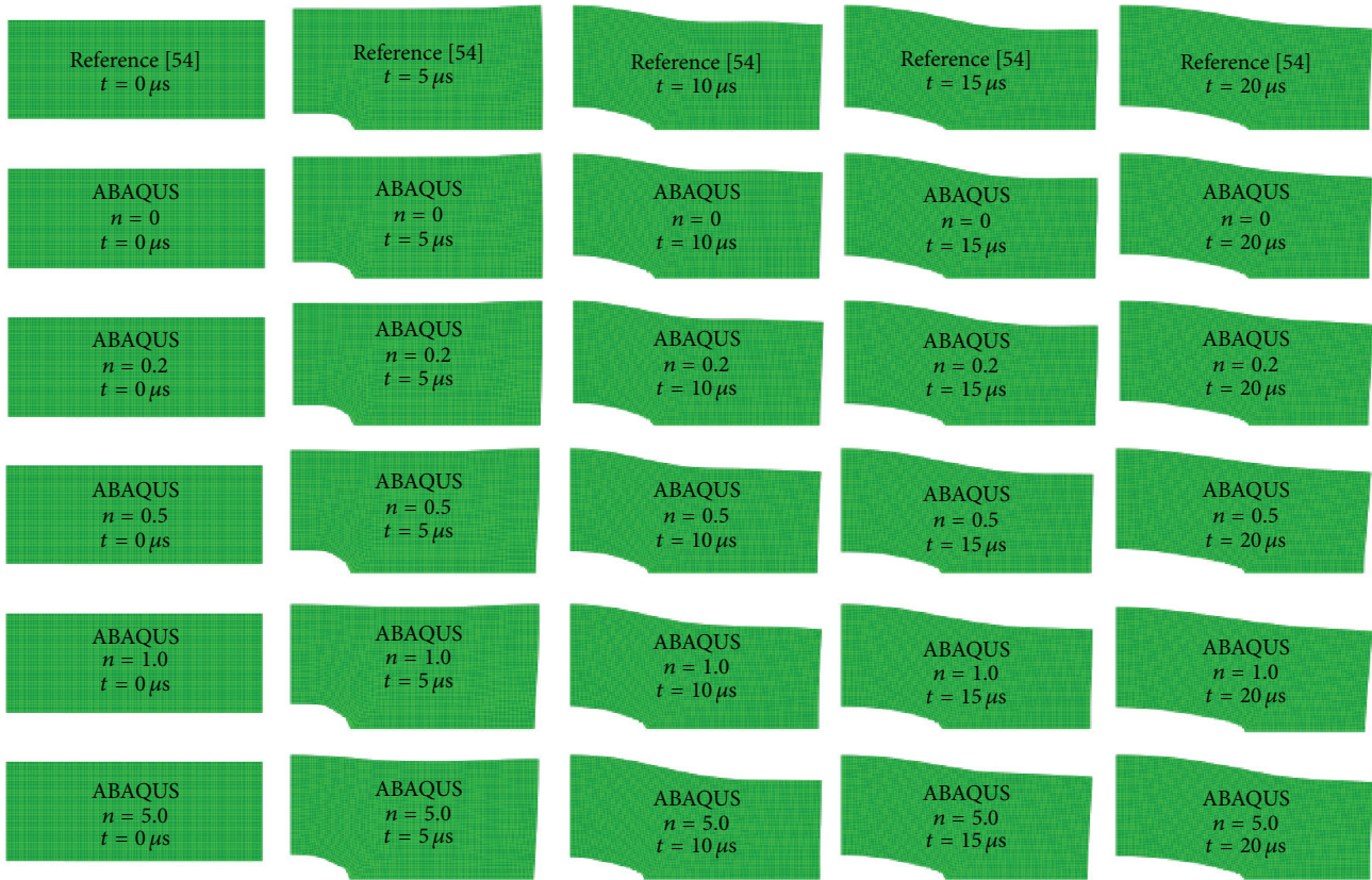
FIGURE 13: Deformed body for dynamic crack propagation at different crack length ( C = 1000 m/s).
